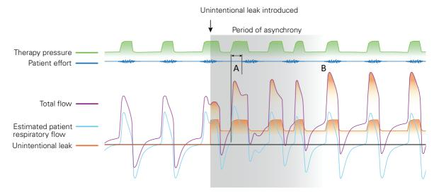
Unintentional leak flow varies with changes to therapy pressure or the size of the leak opening. Vsync calculates changing leak by:
