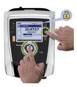
To activate Clinical mode ①, hold down ② and ③ simultaneously for at least three seconds. You will be prompted for how long the device should stay in this mode. After the set period of inactivity or next power cycle (power on/off), the device automatically switches back to the patient mode and the device beeps.
