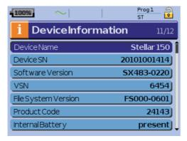
This screen shows the serial number (displayed as Device SN), software version and other component versions. Data on this screen may be requested for servicing or as part of problem-solving by a technician.
