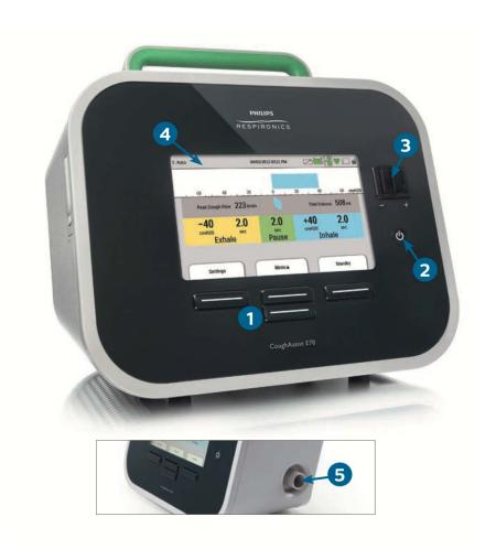
5. Breathing circuit connection. Connect your circuit to the outlet of the device.
