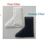
Coarse filter should be WASHED once weekly, CHANGED once yearly. Fine filter CHECKED monthly, CHANGED/DISPOSED minimally every 6 months.
