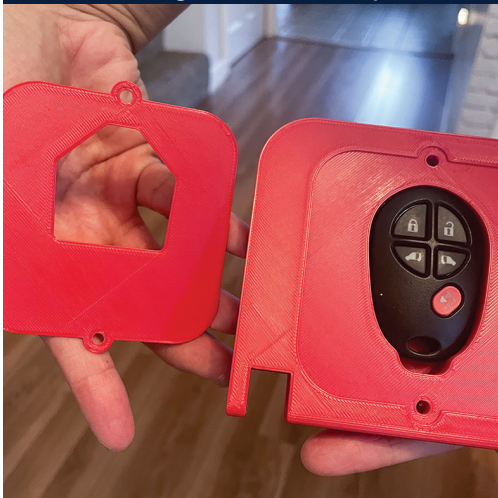
3D printed frame the fob sits snugly inside and will provide enough surface to attach the SwitchBots.
